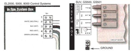
1. To gain access to the spa's control box, remove the cabinet panel on the front of the spa, under the spas topside control. After removing the cabinet panel, remove the four metal control box cover screws and cover. (Two screws on GS500 Pack)
